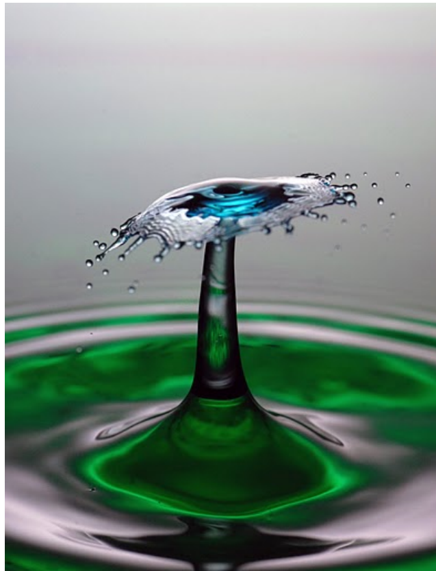
Figure ??. SPOT strobe, Nikon D200, Tamron 90mm macro lens, f/14, 400ISO, colored water and glycerin. 105 ms flash delay, 110 ms droplet delay, 5100 us droplet formation time.
