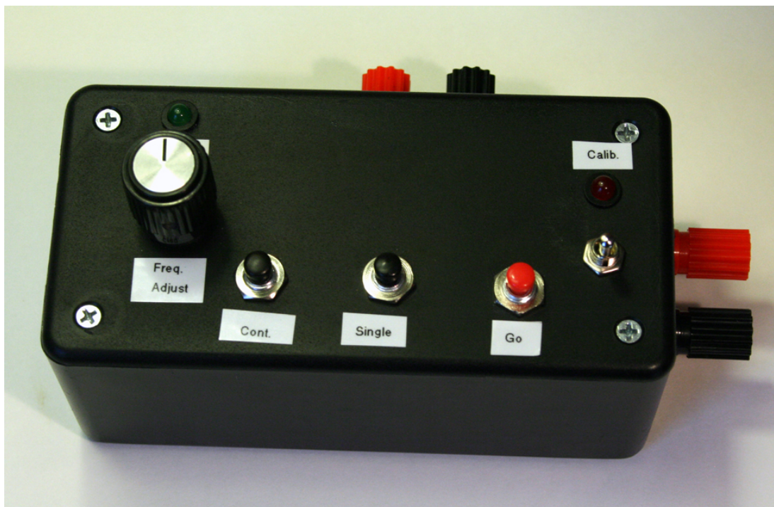
Figure 6. Droplet controller for timing droplets, performing pump maintenance, and calibrating the droplet collider. The connections to the right are for the 100V power supply, and the connections at the back of the device (top of the photo) are for the solenoid pump.
