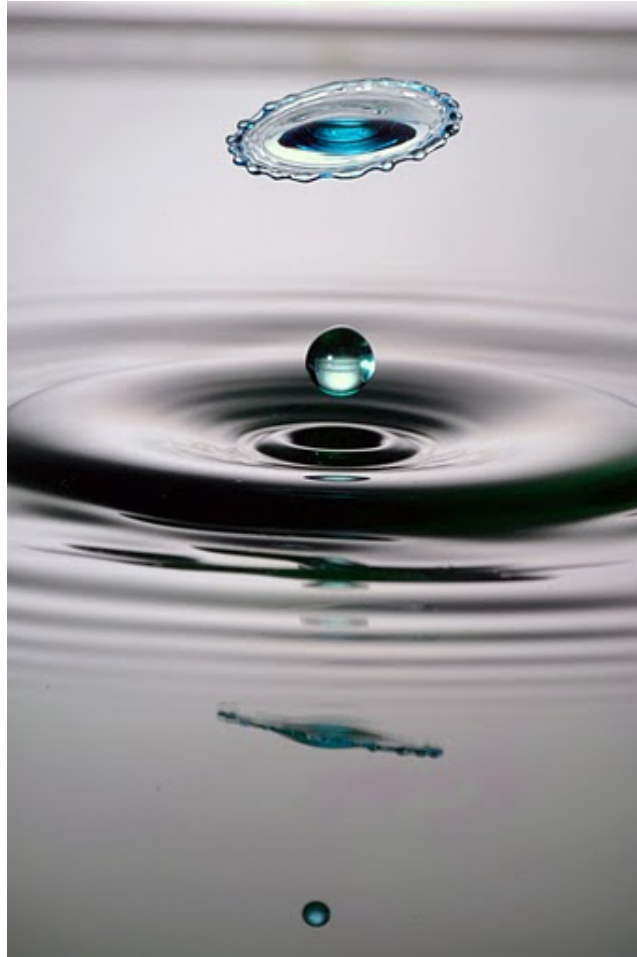
Figure ??. SPOT strobe, Nikon D200, Tamron 90mm macro lens, f/25, 800ISO, colored water and glycerin. 173 ms flash delay, 179 ms droplet delay, 5260 us droplet formation time.
